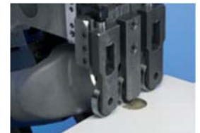
Nested top fine trim with 3 roller tracing.
